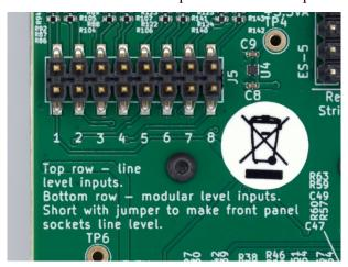
Instructions are printed on the PCB. Fitting a jumper across the pins for a particular input makes the front panel socket line level instead of modular level.
