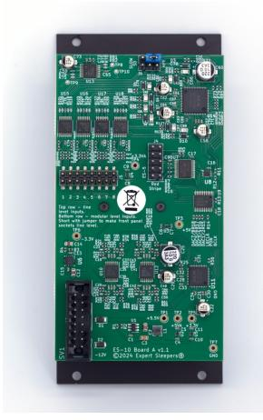
The ES-10 is a Eurorack 8-in/8-out ADAT interface, with DC-coupled inputs and outputs that can be used for both audio and CVs.
