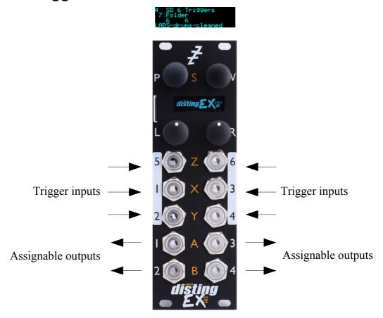
This algorithm, primarily designed for drum sample playback, offers 6 voices with independent triggers and sample selection.
