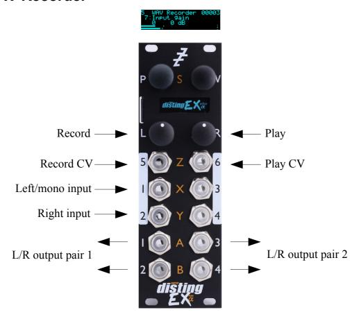
This algorithm records audio (or CV) to the MicroSD card as a WAV file. It can record mono or stereo files at 48 or 96kHz, 16 or 24 bit. It can also play previous recordings, though the various WAV playing algorithms offer many more possibilities.
