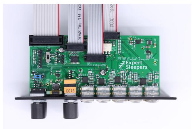
House the module in a Eurorack case of your choosing. The power connector is <u>Doepfer standard</u><sup>1</sup>. If using the power cable supplied with the module, the red edge of the cable is furthest from the top edge of the PCB, and carries -12V. ("-12V" is marked on the PCB itself next to this end of the connector.) Be sure to connect the other end of the power cable correctly, again so -12V corresponds to the red stripe on the cable.
