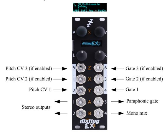
The SD Multisample algorithm is an 8 voice polyphonic sample playback instrument, playing WAV files from the MicroSD card. It can have up to 3 input CV/gate pairs, or can be played via MIDI. It supports both velocity switches and round robins per sample.
