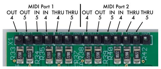
Pin numbers refer to the 5-pin DIN socket as in the MIDI specification<sup>2</sup>.
