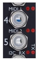
The three pairs refer to the three channels of communication – MIDI 1, MIDI 2, and I2C. For each pair the left LED indicates that the module is receiving, and the right LED that the module is transmitting.
