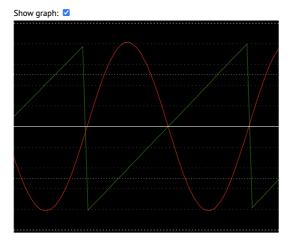
Each input is shown in a different colour – red, green, blue, cyan, magenta, yellow, orange, and white for inputs 1 to 8 respectively.
